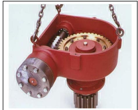
The intermediate worm gear housing is cast iron, flange-mounted to the cast iron spur gear housing with a full 360 degree bearing area. At least one competitive brand does NOT
