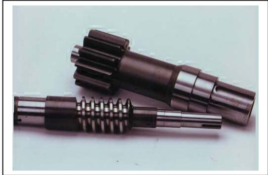
The subject of aspect ratio is new to ANSI/AGMA standard 2001. Specifically it relates the drive rating to the aspect ratio; higher aspect ratio, which by definition results in a weaker, less rigid pinion with resulting mesh misalignment, demands downrating the torque capacity. Walker Process drives have among the lowest, if not the lowest, aspect ratios in this industry.
